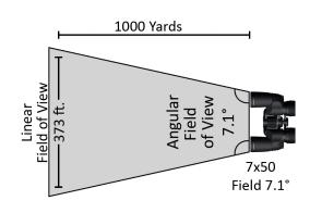
Multiply the angular field by 52.5' to determine the linear field. A 7.1 degree angular field has a 373' linear field at 1,000 yards in front of you.
